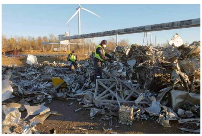
Customs officials inspecting a scrap metal load using radiation monitoring equipment in Tornio in October 2018.
